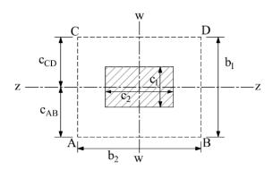
Critical shear perimeter for interior column
