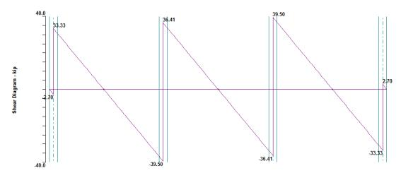
Shear Force Diagram from spSlab
