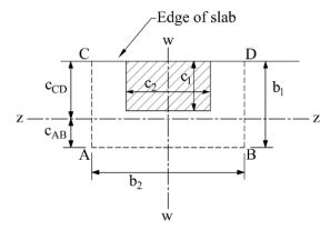
Critical shear perimeter for exterior column
